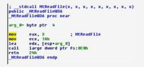
Working with Windows XP and higher, we only have to implement three call gates. We'll do so in an inline assembly within our C++ code like so:
